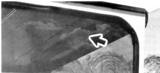
FIGURE 12. Damaged Cab Window.
