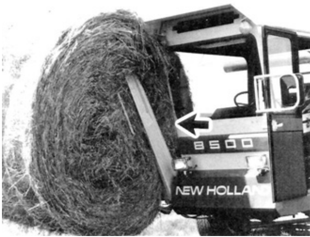
FIGURE 2. Bale Interference with the Operator's Cab while Loading 72 in (1830 mm) Soft Core Hay Bales.
