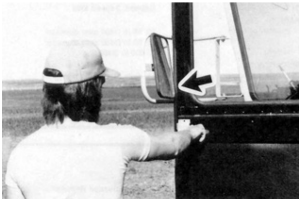
FIGURE 7. Interference between Rear View Mirror and Cab Door.
