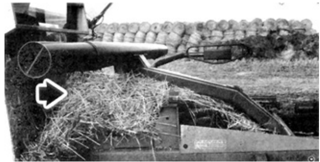
FIGURE 8. Collection of Loose Material below Pusher.
