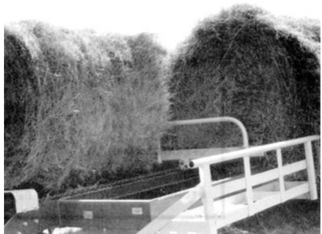
FIGURE 4. Bale Drag Trapped Between Bales.
