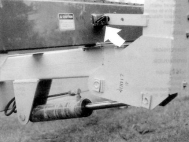
FIGURE 4. Lift Arm Safety Lock Pin.
