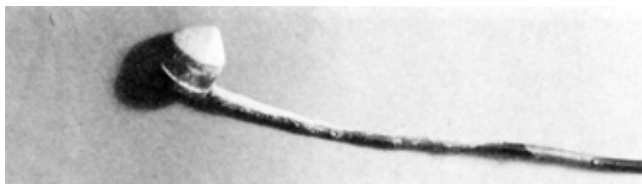
FIGURE 3. Powder Buildup on Sensor Face.
