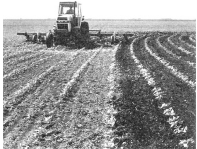
FIGURE 6. Normal surface left by cultivator.
