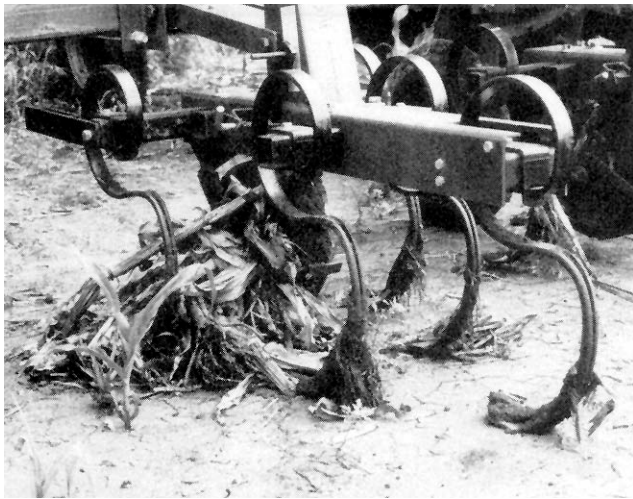
FIGURE 5. Plugged gang due to gauge wheel interference.
