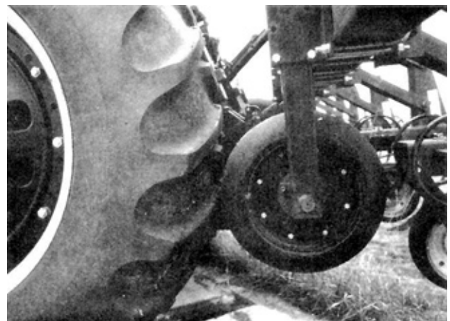
FIGURE 8. Interference between tractor tire and cultivator.
