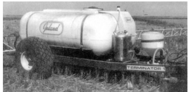
FIGURE 6. Foam Tank and Compressor Housing.
