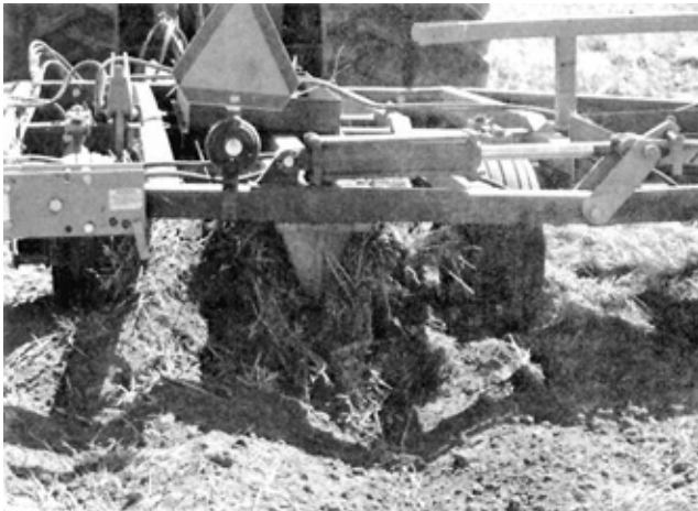
FIGURE 5. Plugging at the Centre Shank.
