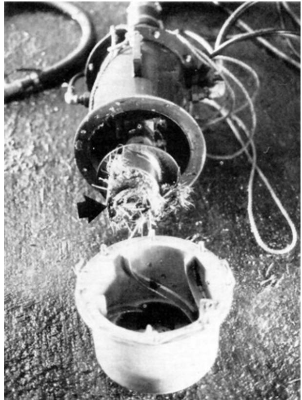
FIGURE 5. Straw Plugging the Impeller Centre.
