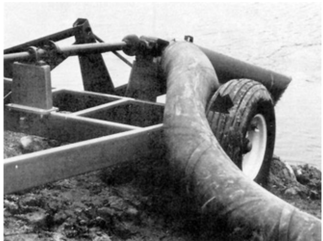
FIGURE 5. Improper Discharge Hose Placement Resulting in a Discharge Restriction.
