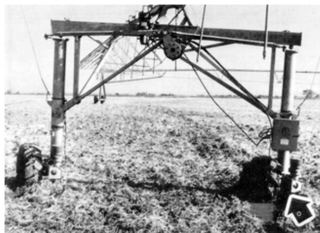
FIGURE 19. Broken Flexspan Corner Attachment Tower Axle.
