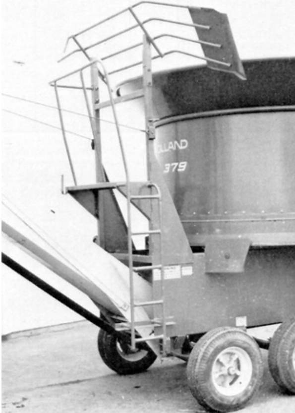
FIGURE 9. Guide Rack and Winch Cables.
