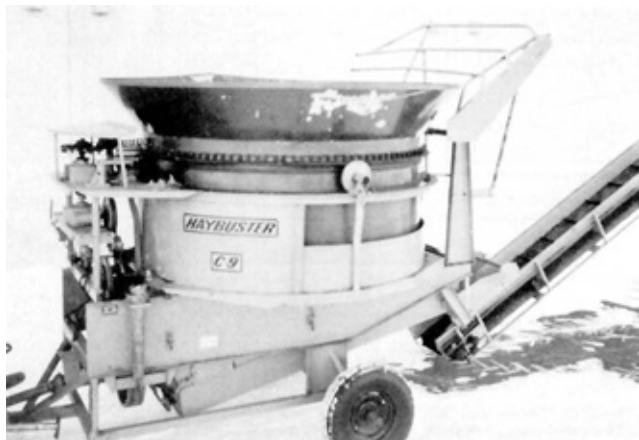
FIGURE 3. Tub and Guide Rack.
