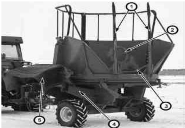
Figure 1. (1) Bale forks, (2) Tub/Chamber, (3) Bale driver arms, (4) Distribution chamber,
