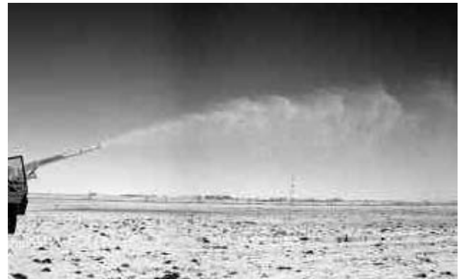
Figure 4. Highline Top Gun distributing dry straw at the maximum height.
