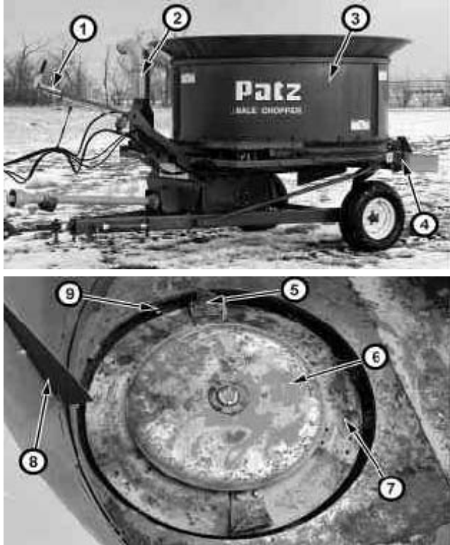
Figure 1. (1) Flow control system and lever, (2) Front high right discharge spout, (3) Tub/Chamber, (4) Low rear left discharge port, (5) Upright cutting knives, (6) Center hub, (7) Processing rotor, (8) Bale grippers, (9) Fan blades.
