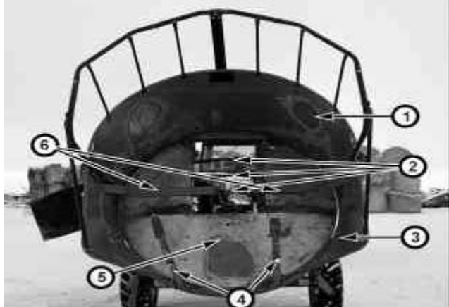
Figure 2 a. (1) Tub/Chamber, (2) 3 Grid bar rotor guards, (3) Chamber hydraulically tilted 90°, (4) Bale lifting forks, (5) Tub floor, (6) Bale driver arms.
