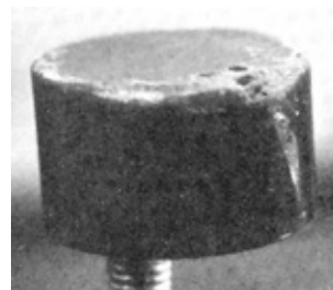
FIGURE 10. Damaged Speed Sensor.
