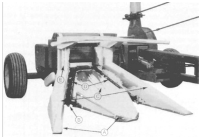
FIGURE 3. Two-Row Row Crop Head: (A) Divider Noses, (B) Oscillating Knife, (C) Nose Adjusting Straps, (D) Gathering Belts, (E) Gatherer Feedroll.
