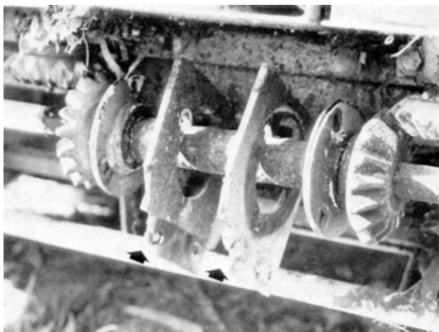
FIGURE 8. Broken Bearing Supports.
