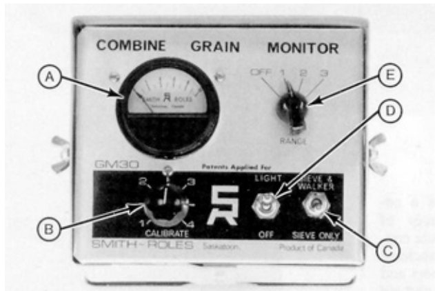
FIGURE 3. Control Box: (A) Loss Meter (B) Calibration Control (C) Sensor Selector Switch (D) Meter Illumination Switch (E) Power Switch and Meter Range Control.
