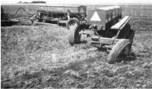
FIGURE 12. Disk Harrows Midway Through a Left Turn.
