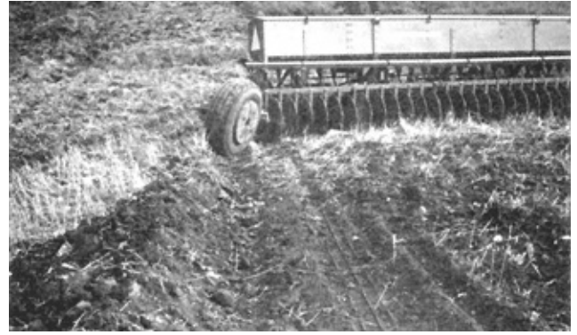
FIGURE 4. Rear Furrow Wheel Leaving the Furrow when Operating Downhill.
