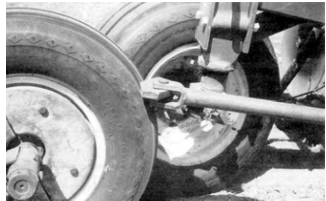
FIGURE 17. Interference Between Furrow Wheel Steering Arm and Rear Furrow Wheel when Placing into Full Transport with the Disk Gangs Raised.
