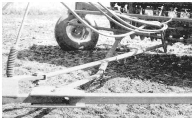
FIGURE 21. Buckled Hitch Brace.
