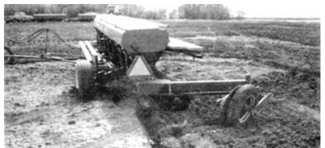
FIGURE 15. Skidding of the Rear Land Wheel when Making Sharp Left Turns.
