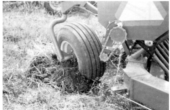
FIGURE 14. Skidding of the Locked Rear Land Wheel when Making Left Turns Greater than 90°
