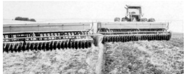
FIGURE 5. Centre Furrow Wheel Leaving the Furrow when Width of Cut Exceeds 9.2 m.
