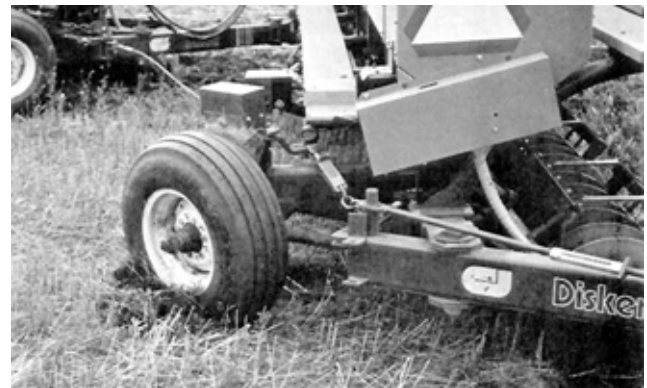
FIGURE 11. Skidding of the Rear Land Wheel when Making Sharp Left Turns.
