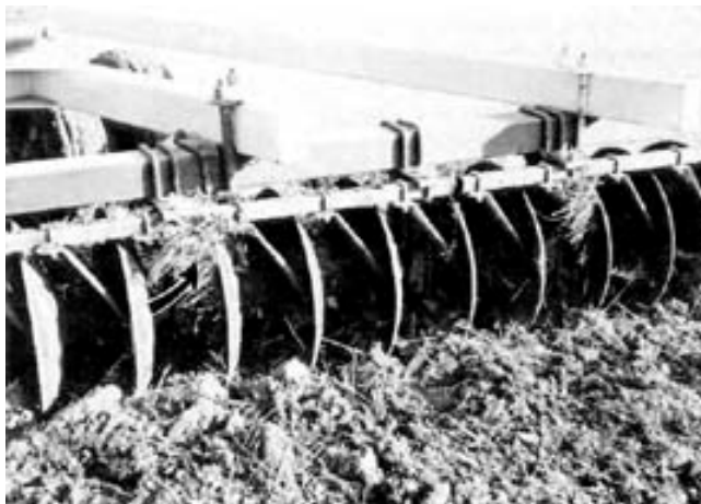
FIGURE 2. Trash Buildup Between Scrapers and Gang Bearing Hangers.
