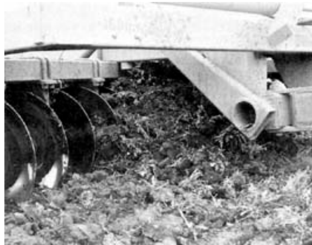
FIGURE 3. Plugging at the Center of the Front Gangs.
