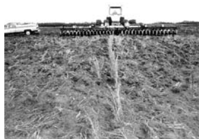
FIGURE 6. Weed Misses Caused by Stripping in the Center.
