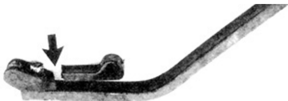
FIGURE 12. Broken Shank Attaching Casting.
