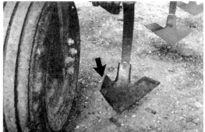
FIGURE 10. Sweep Wing Cut-off to Prevent Tire Damage.
