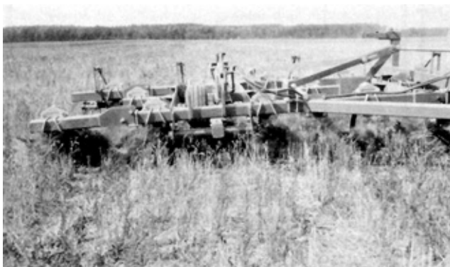
FIGURE 5. Excessive Wing Penetration in Heavy Primary Tillage.
