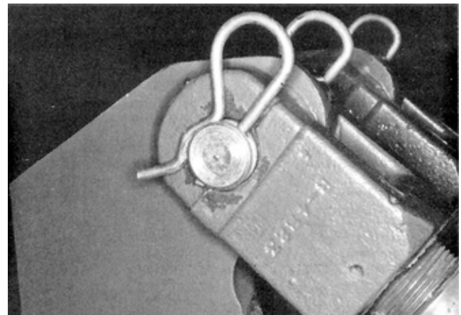
FIGURE 13. Damaged Retainer Clips on Cylinder Yokes.
