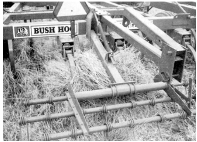
FIGURE 5. Plugging Between the Centre Shanks and Finishing Harrows.
