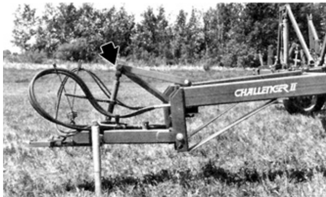
FIGURE 10. Hitch Height Adjustment.
