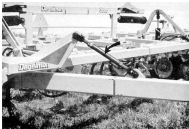
FIGURE 9. Hitch Height Adjustment.
