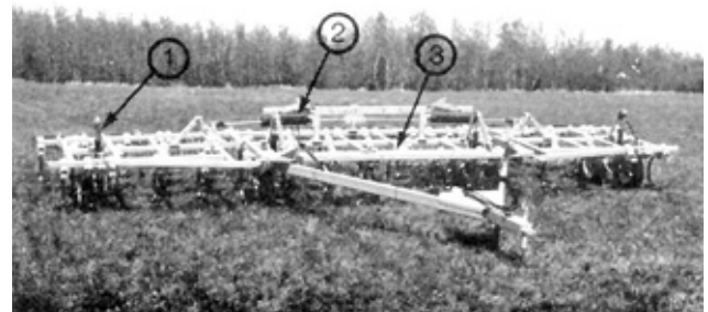
FIGURE 1. Degelman 3000 (1) Depth Control Cylinders, (2) Wing Lift Cylinders, (3) Hydraulic Flow Divider.
