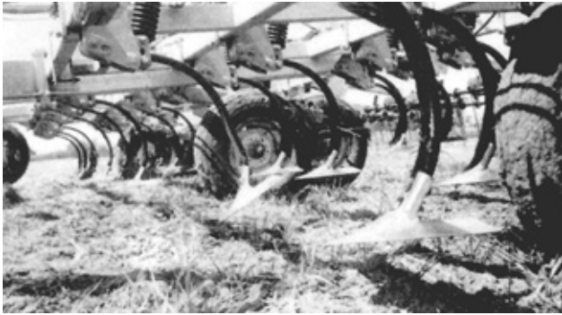
FIGURE 11. Shank Bent After Contacting the Frame.
