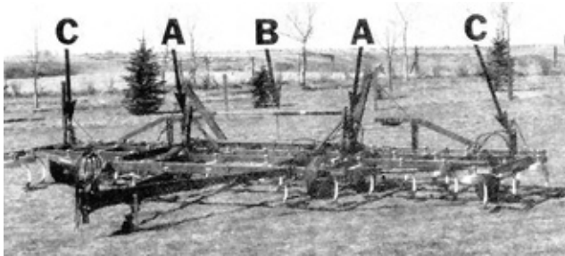
FIGURE 1. International 645: (A) Master Cylinders, (B) Wing Lift Cylinder, (C) Slave Cylinders.
