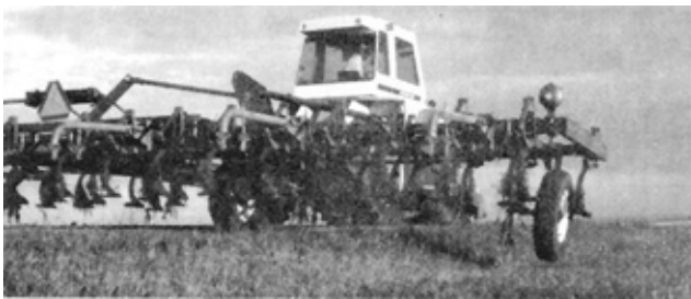
FIGURE 5. Wing Lift Linkage Preventing Wings Pivoting Downward in Relation to Centre Frame.
