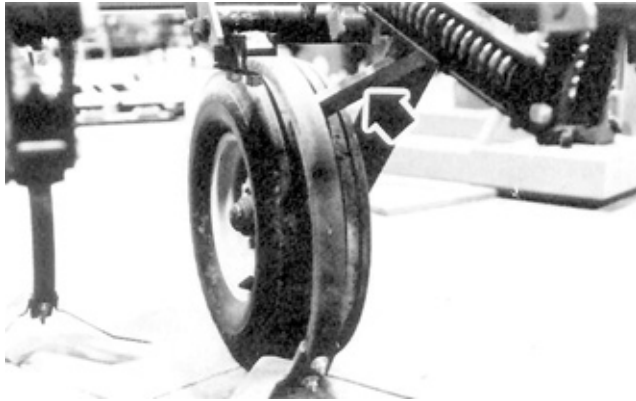
FIGURE 6. Stop Bar Preventing Release of Shanks Adjacent to the Wheels.
