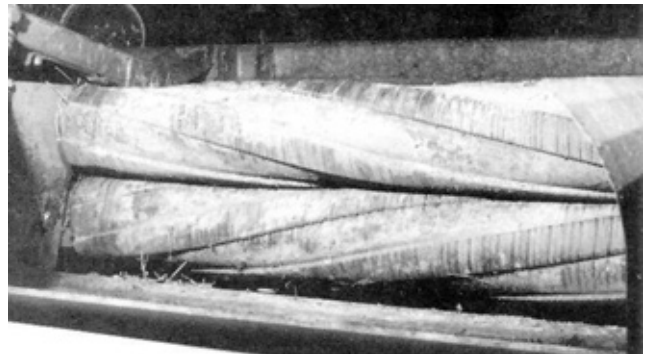
FIGURE 6. Conditioner Rolls Showing Signs of Wear.
