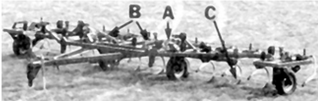
FIGURE 1. Edwards GN-R78-436: (A) Master Cylinder, (B) Wing Lift Cylinders, (C) Cultivator Shanks.
