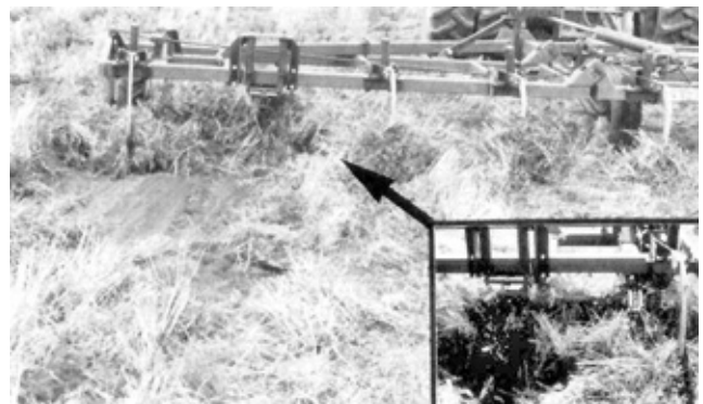
FIGURE 4. Plugging at the Wing Section Drive Shafts.
