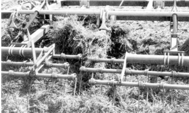
FIGURE 4. Plugging at the Wing Wheel Location in Heavy Trash.
