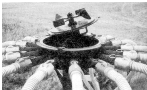
The slurry distribution manifold has a hydraulically powered, rotary cutting/distribution system.
