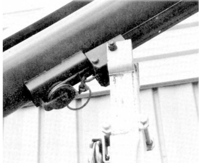
FIGURE 2. Cable Interference at 30° elevation.
