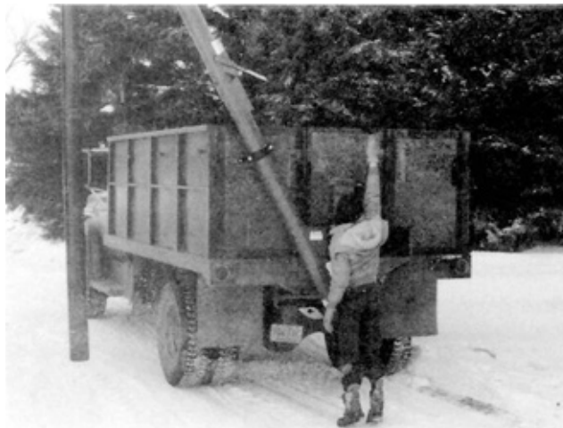
FIGURE 5. Folding Lever Difficult to Reach.
