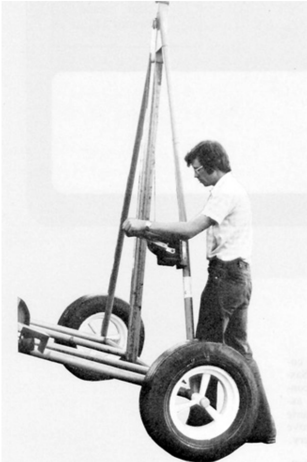
FIGURE 2. Inconvenient Winch Handle Location.
