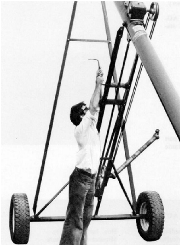
FIGURE 2. Inconvenient Winch Handle Location.
