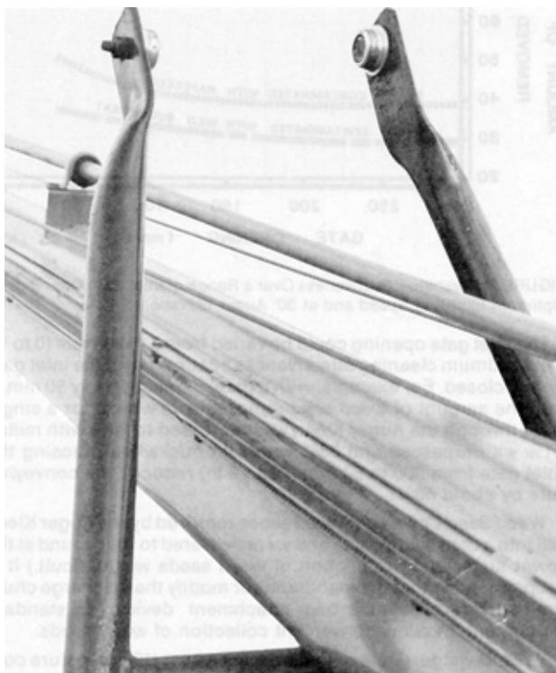
FIGURE 11. Damage to Conveyor Tube Front Supports when Attempting to Raise the Auger Kleen higher than 30°.
