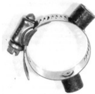
FIGURE 5. Modifications to Hose Clamp Pickup to Increase Signal Strength.
