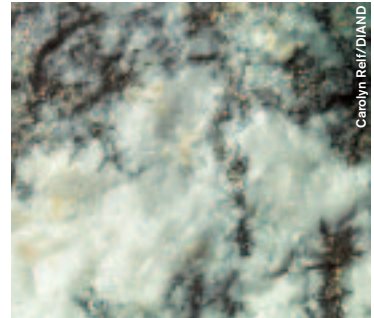
Mineralized sample contains gold, silver, pyrite and quartz.
