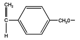
serves as raw material for a setting resin when mixed with unsaturated monomer and cured (addition reaction).
