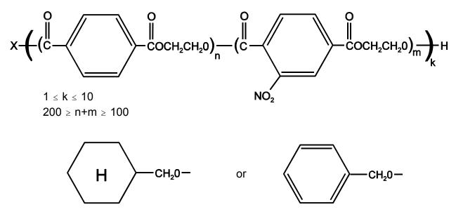
All of the above copolymers have in common a thermal degradation resistance property, due to the reduced number of free COOH radicals by esterification with X of the end COOH radicals which cause thermal degradation. The chemical structures of the alternatives are considered to be technically closely interrelated to one another. A grouping in one claim is therefore allowed.
