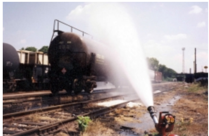
A rail tank car of Butanol being cooled by a fire department during an emergency response.
