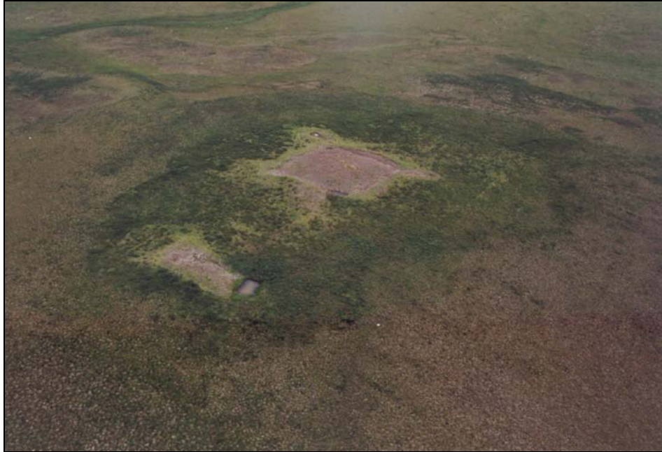
Figure 8. An intact sump (Gulf Mobil Ogeoqueoq J-06) in the Parsons Lake area. Note that the sump cap is largely unvegetated and that the site is well-drained. Photograph: Summer 2000.
