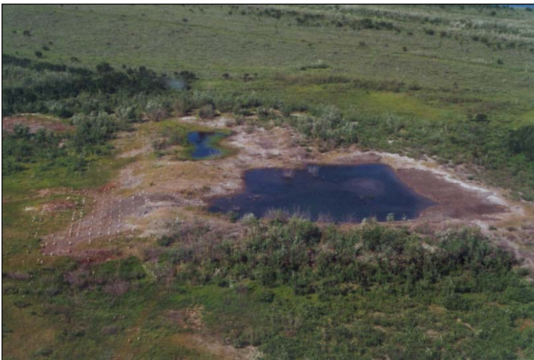
Figure 5. Salt efflorescences and dead vegetation around the sump perimeter in Mackenzie Delta (Shell Kugpik O-13) indicate contamination of surrounding terrain. Contaminants are slowly flushed from these sites by floodwaters of the Mackenzie River. Photograph: Summer 2000.
