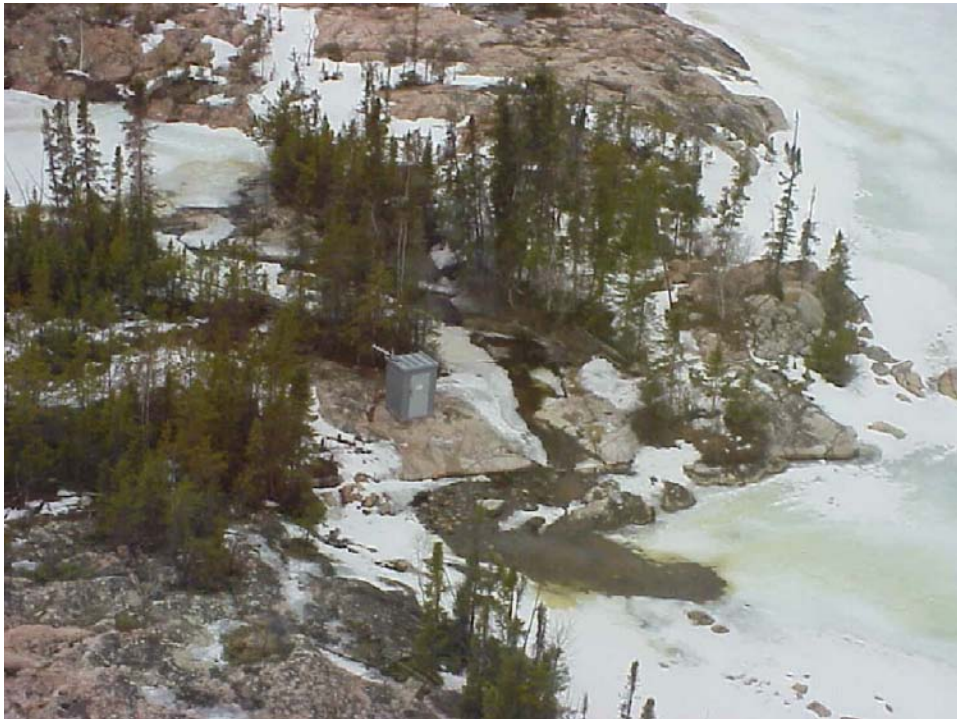
Photo 2. Hydrometric gauge at Baker Creek at outlet of Lower Martin Lake (Photo: Water Survey of Canada (WSC), Yellowknife NT)
