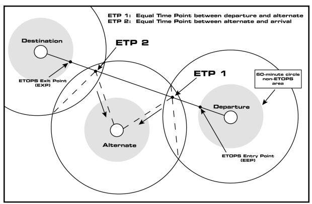
Established earliest time of landing: High speed cruise (2 engine operating and high altitude) from ETP 1 to alternate.
