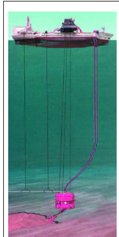
Figure 5.2 Remotely Operated Dredging Unit
